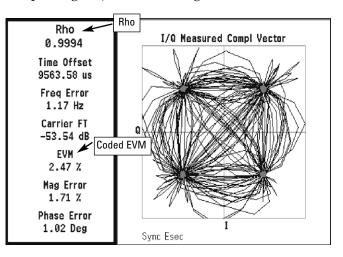
Figure 9. Rho and coded EVM measurement on a cdma2000 SR1 pilot signal
