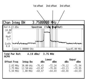
Figure 5. ACPR measurement for a cdma2000 SR3 DS signal
