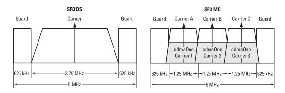
Figure 2. Bandwidth limits for SR3DS and SR3 MC
