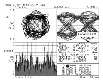
Figure 13. EVM (uncoded) on a cdma2000 SR1 reverse link signal with R-Pilot and R-FCH (RC3 at 9.6 kbps) activated. Both channels are at the same power level
