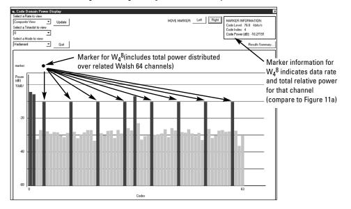
Similar considerations apply to SR3 MC signals. Additionally, in this case an instrument with code-domain power capability for cdmaOne can only make the measurement on a single carrier of the SR3 MC signal at a time.
