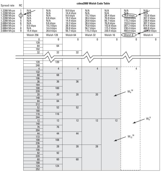
Figure 17. Using  $W_4^8$  precludes the codes in the shaded area.
